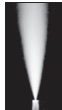
The CPI PFA Micro-Flow Nebulizer produces a fine aerosol for high transport efficiency and high sensitivity.
